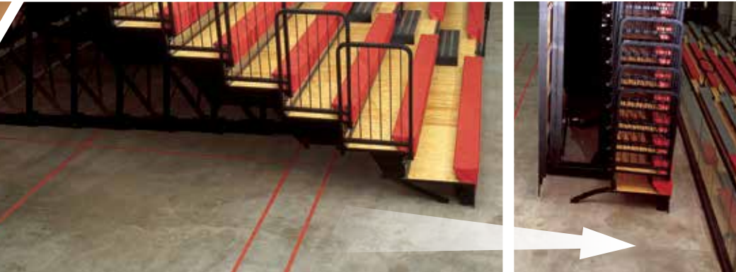
Reverse-Fold Delayed Action Further increase your usable space by up to 3' (914 mm) with MAXAM's delayed action feature. The entire closed bleacher stack moves forward on a linkage to recover additional floor space.
